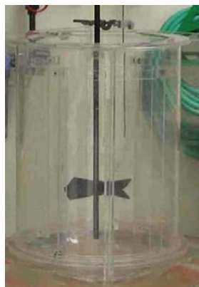
Figure 1: Stir Tank (Courtesy Dow Chemicals)
